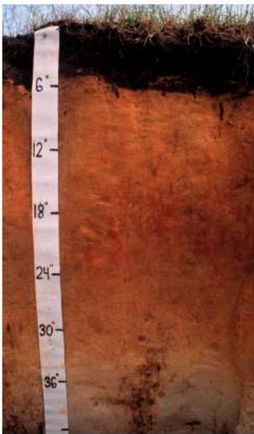
Figure 27.—Typical profile of Seabrook fine sand, 0 to 3 percent slopes, rarely flooded. Most areas of Seabrook soils are in the Grassy Ridge area of Hyde County.
